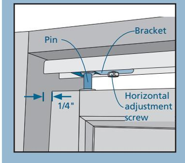
5. Verify there is a 1/4" clearance between the pivot door and the jamb. Four panel assemblies should be snug at the middle. If adjustments are necessary, door panels should be folded, in some cases removed, to gain access to the adjustment screws.
