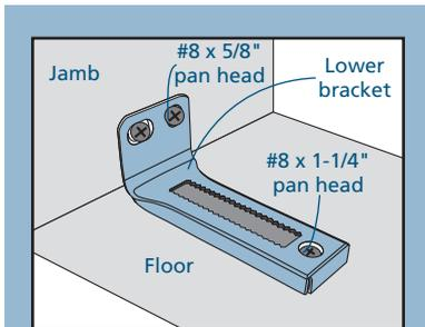
4. Place the upper pivot pin in the hole in the bracket and the guide in the track (or in the middle of the slide guide between the springs). Lift the door assembly slightly and drop the lower pin into the lower bracket slot.
